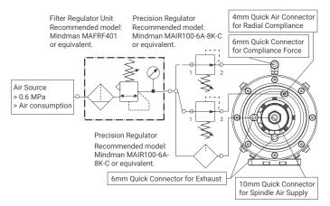
2. Check the CENTER POINT (\*1) first, giving 0.2 MPa pressure to the compliant force connector while the spindle is turning off. Make sure the spindle is able to return to the CENTER POINT as shown as the illustration below. Please contact your supplier if it couldn't return to or is not on the CENTER POINT.
