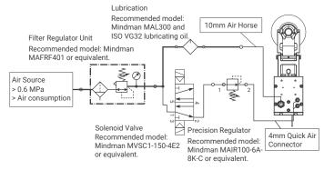
Check the CENTER POINT (\*1) first; giving 0.2 MPa pressure to the compliant force connector while the spindle is turning off. Make sure the spindle is able to return to the CENTER POINT as shown as the illustration below. Please contact your supplier if it couldn't return to or is not on the CENTER POINT.
