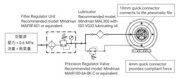
2. Check the CENTER POINT (\*1) first; giving 0.2 MPa pressure to the compliant force connector while the spindle is turning off. Make sure the spindle is able to return to the CENTER POINT as shown as the illustration below. Please contact your supplier if it couldn't return to or is not on the CENTER POINT.
