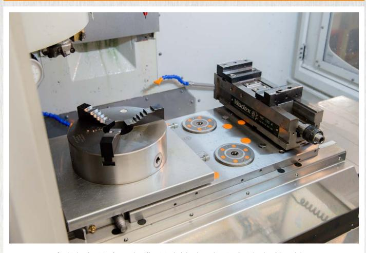
8-point clamping station for mounting different standard clamping equipment or direct clamping of the workpiece.
