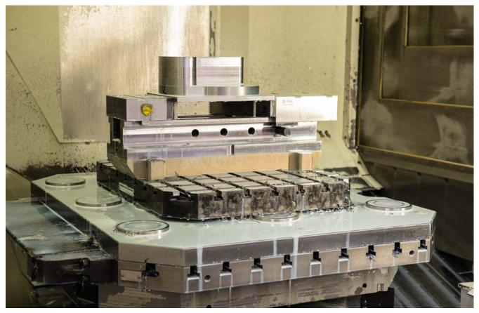
Thanks to the low installation height of our clamping modules, the assembly of the clamping device can be adapted flexibly to the respective machining height and workpiece
