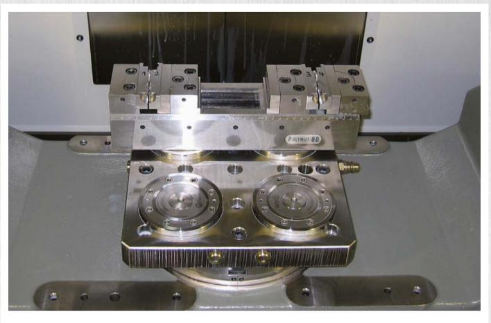
The 4-point clamping station replaces the machine table. This guarantees maximum utilisation of the machine's stroke.
