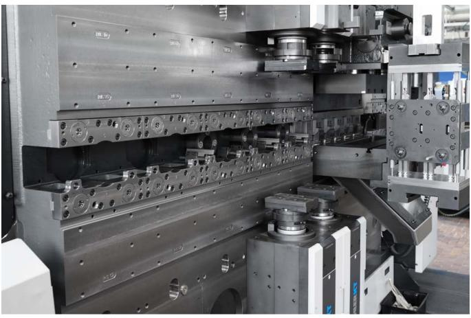
Each receptacle is equipped with four zero-point clamping modules. Thanks to the compact design, the clamping modules can screwed in easily and flush.
