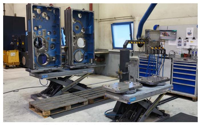
Lifting tables equipped with zero-point clamping technology for deburring the workpieces. As a result, the complete manufacturing process has been seamlessly optimised with the AMF Zero-Point-System.
