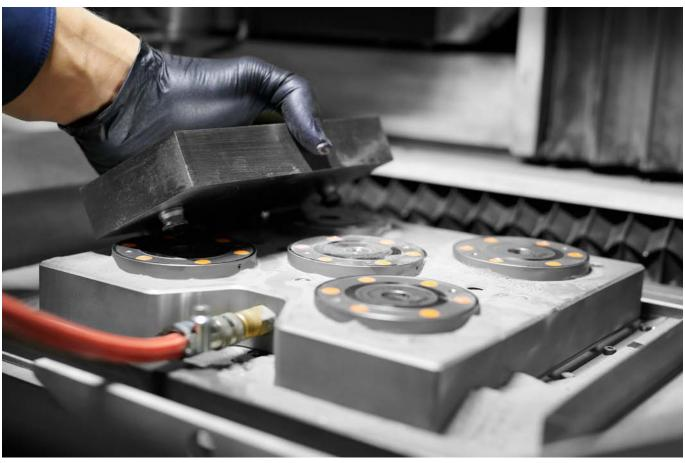
AMF-Zero-Point-Systems in additive manufacturing.
