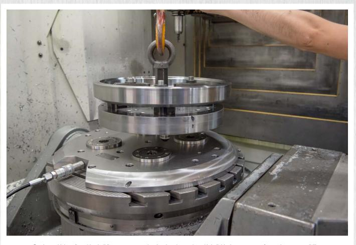
5-axis-machining of machine building components. 4-point clamping station with individual outer contour for maximum accessibility.
