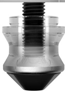
> The pull-stud in our zero-point system is the interface between the machine table and the workpiece or fixture. It ensures exact positioning and secure clamping. The resulting work forces are transferred through the pullstud to the clamping module.
