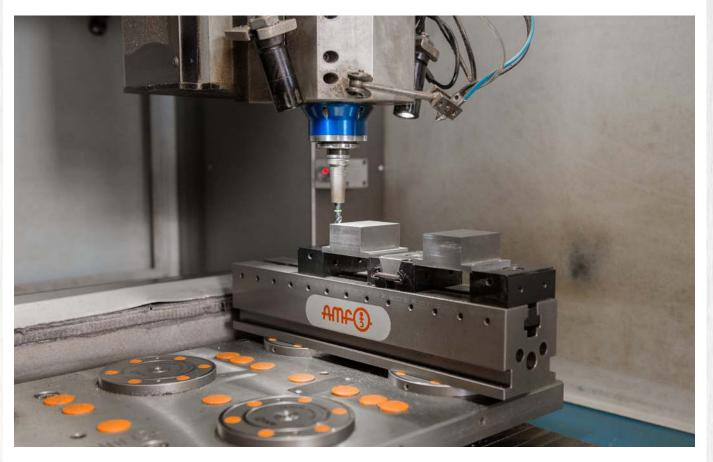
$\ensuremath{\mathsf{AMF}}$  multiple clamping system in conjunction with the  $\ensuremath{\mathsf{AMF}}$  zero-point system.
