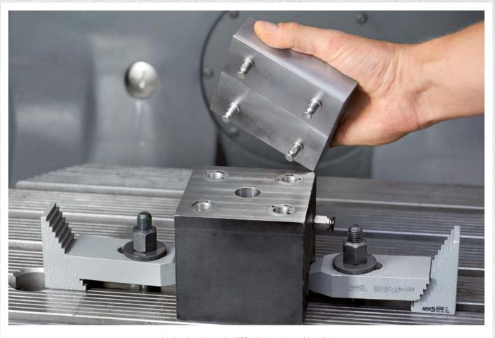
$\hbox{4-point clamping station KO2 with interchangeable pallet}.$
