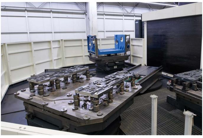
The zero point clamping towers are flexibly adapted to the respective workpiece by simply repositioning them.
