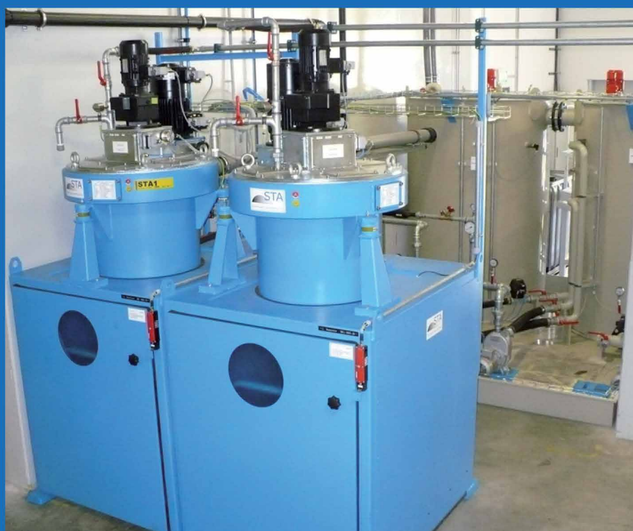
Central system for 3.000 lpm grinding emulsion
